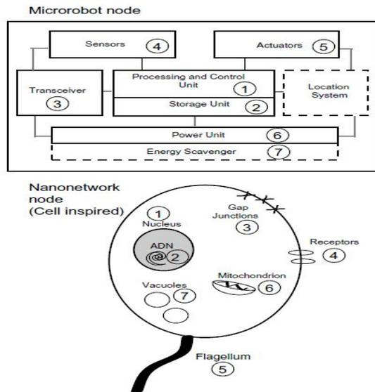
**Fig. 2. Functional architecture mapping between nano-machines of a micro or nano-robot, nano-machines found in a cell**
