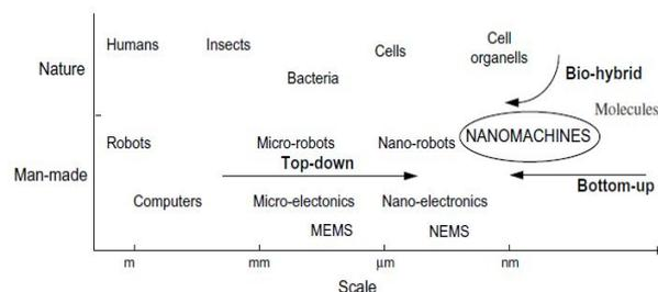
**Fig. 1. Approaches for the development of nano-machines**
